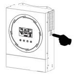
Step 4. Be sure to select battery type as "SOL" in LCD program 5.
